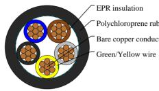
Polychloroprene rubber outer jacket Bare copper conductor
